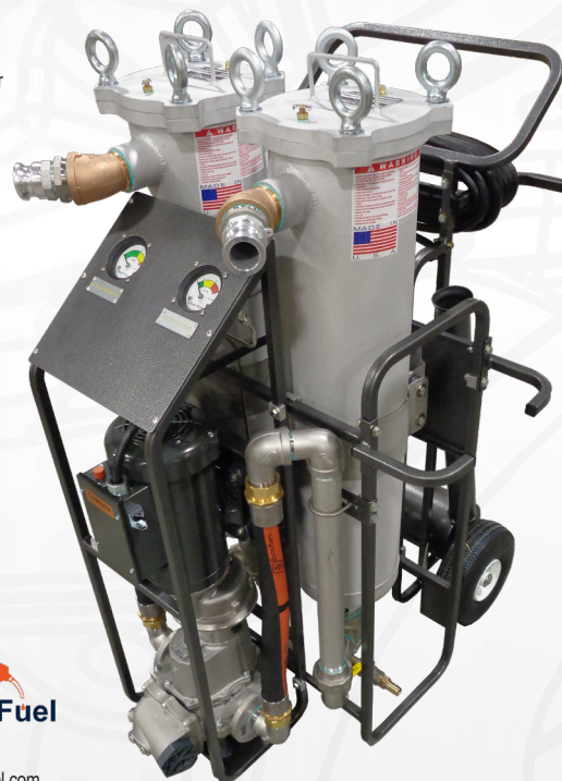
FS2 Mobile Filtration - 35 GPM - 2-Wheel Dolly - Inlet: Bag Filter, Outlet: Coalescing/Water Separation/Cartridge Filter
